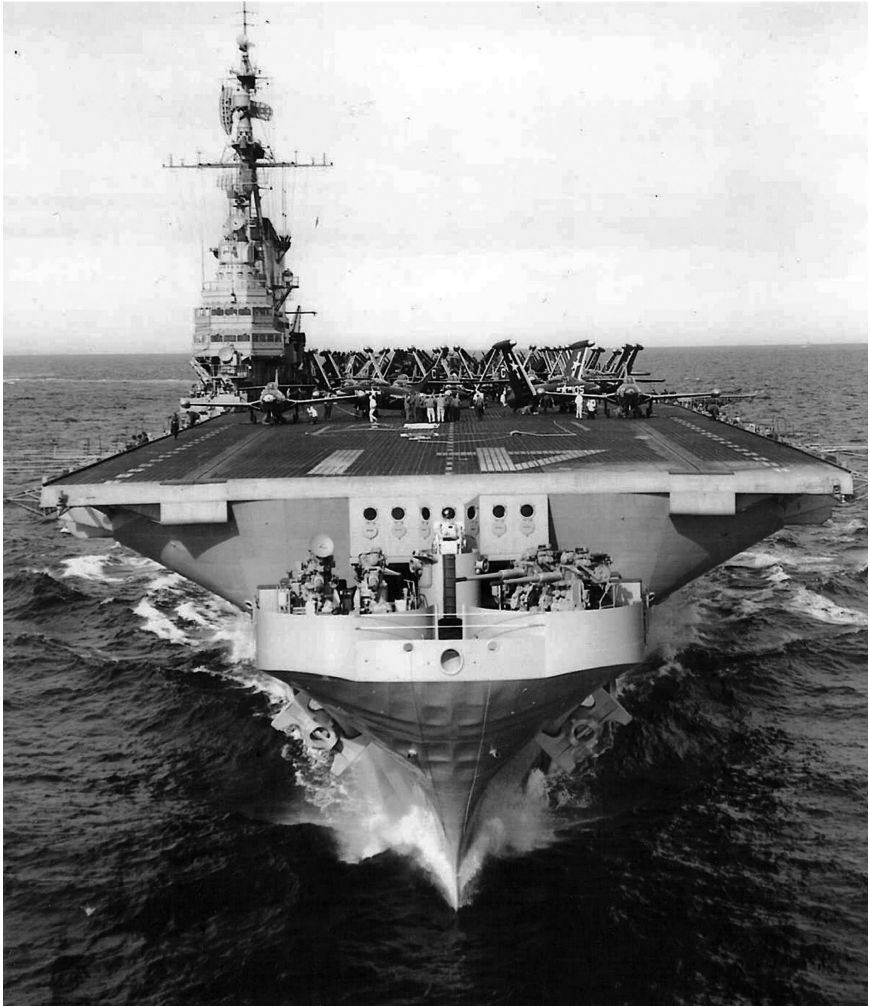
The USS Midway returned to Norfolk, Virginia after a deployment to the Mediterranean in 1951. Note the single “straight deck” and the anti-aircraft guns on the bow. The carrier’s angle deck was added in 1955-57.
